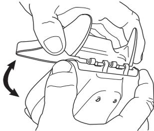
**Important!** Do not open the Aeroclam halves any more than shown above as separating the top and bottom sections will become difficult.
