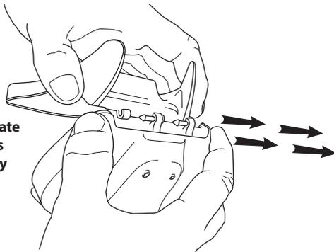
To fix the Aeroclam to your saddle you must separate the Aeroclam halves. Hold the top section in your left hand and slide the bottom section directly away from you with your right hand. **DO NOT TWIST OR WENCH SIDWAYS** as you may damage the hinge.
