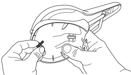
Take the clam top section in the same hand & line the mounting slot up with the nut in the clam then **loosely tighten** the bolt [must use washer!].
