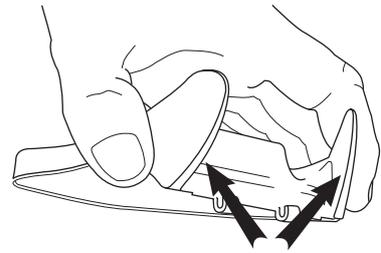
You may need to apply slight leverage to the Style Fins located on the front top section of the Aeroclam to be able to slide past your seat post clamp if it's a wider version.
