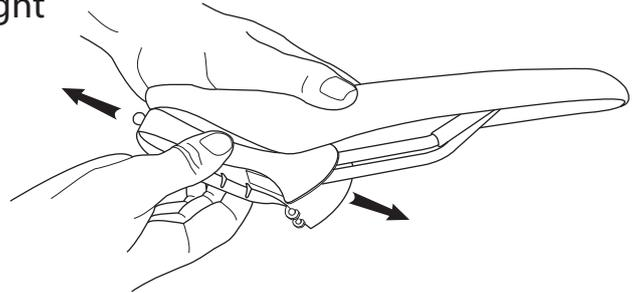
Slide the clam top section backward and forward until it sits at it's most natural position [the Sweet Spot], then tighten. **Do not brutally over tighten!** Firmly is enough. The nylock nut will ensure the clam stays tight.
