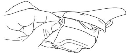
Ensure to properly secure the rubber latch over the buttons by using a pinching motion with forefinger and thumb. Check and retighten bolt after some use.
